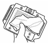
14. Use a dry disposable towel to gently press down on each spring pin (1) on the pluggable heater.
